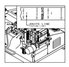
3 Adjust the sensor with guide-control bolt for lightening the beam on the center of marking point.
