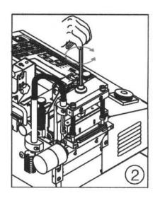
3 Take off the heater after unscrewing the fixing bolt by 4~5mm-wrench. (Install new upper knife and assemble it again vice versa.)
