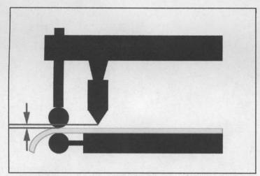
As you can see left image, the upper front feeding roller is lower than hot-knife.
