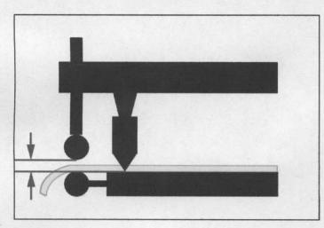
As you can see left image, the upper front feeding roller is higher than hot-knife.
