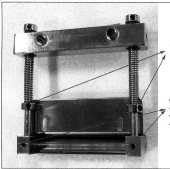
These tow bolts are used when you adjust the pressure of upper front feeding roller.
