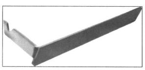
At first, please set the knife's temperature to  $250\,^\circ\text{C} \sim 300\,^\circ\text{C}$  degrees.
